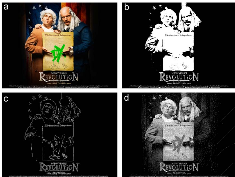
Fig. 1. Image fidelity in different binary representations. Shown, top to bottom and left to right, are original image, graythreshold, edged and dithered versions, respectively. An observer can determine that the dithered version retained most information from the original signal.
