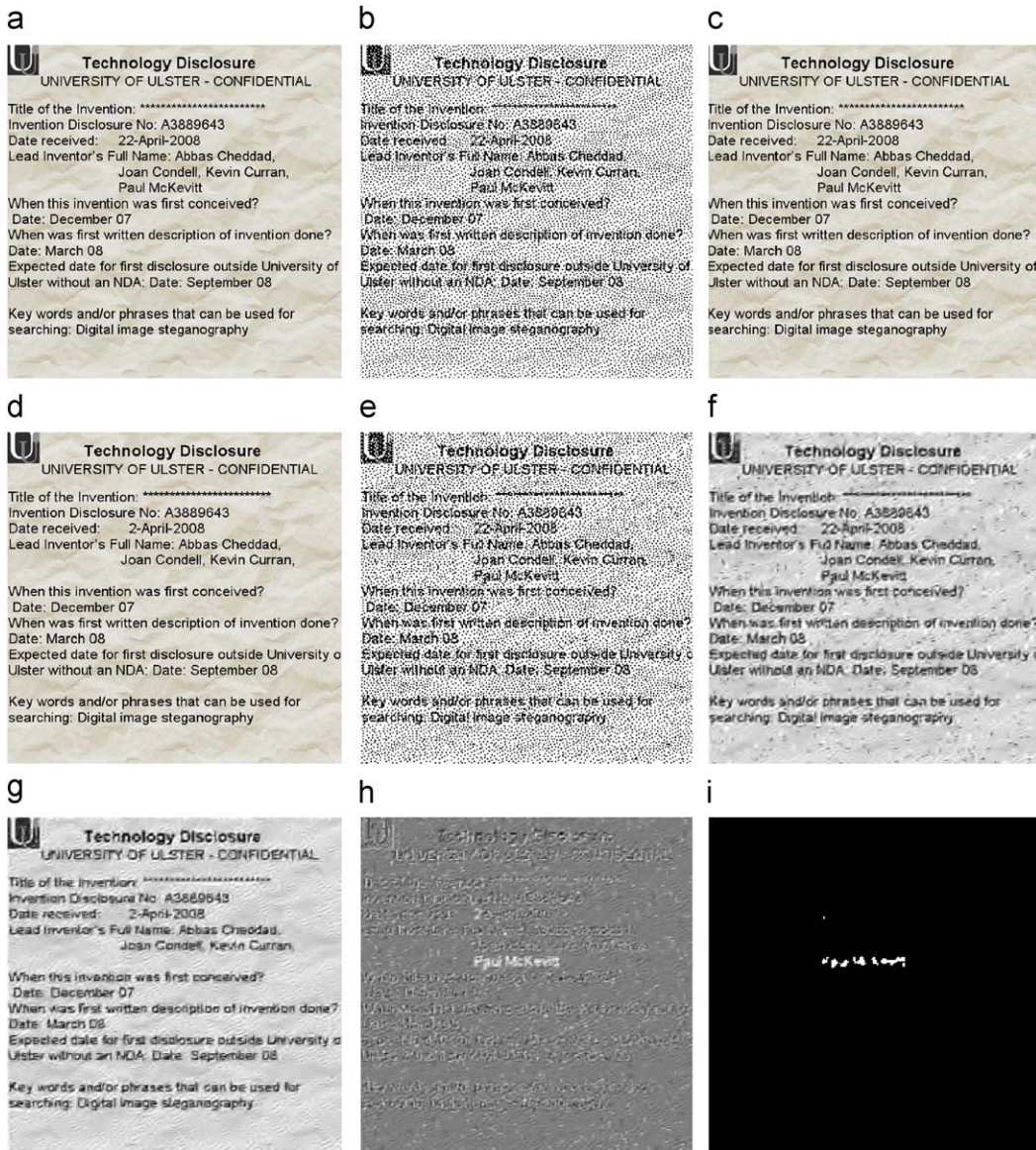
Fig. 7. Example 2, performance of proposed algorithm on digital document: the original document (a), dithered version of original used as a payload (b), Stego-image after embedding (c), attacked Stego, i.e., date received has changed and the fourth lead inventor's name has been removed (d), reconstructed hidden data from the attacked version (e), inverse halftoning of (e) shown in (f), inverse halftoning of (d) shown in (g), error signal of (f) and (g) shown in (h), and (h) after undergoing binary thresholding shown in (i).
