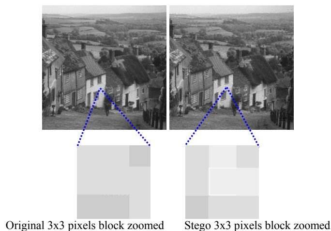
Figure 14: Even though embedding at the DCT level is a very successful and powerful tool. When the coefficients are not carefully selected some artifacts will be noticeable.
